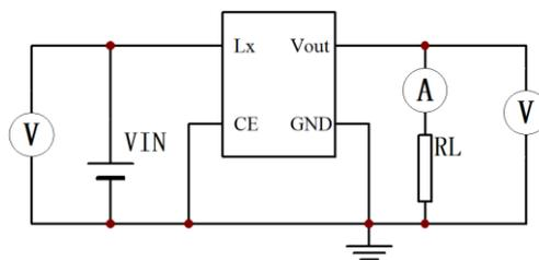
$$R_{OP\_SW} = (VIN - V_o) / I_{out}$$
