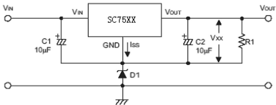
$$V_{OUT} = V_{XX} + VD1$$
