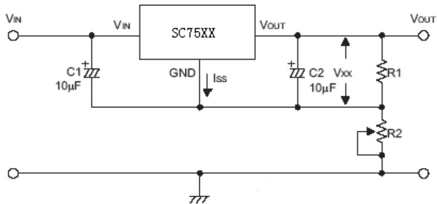
$$V_{OUT} = V_{XX} (1 + R2/R1) + I_{SS} * R2$$
