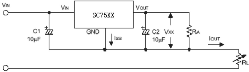
$$I_{OUT} = V_{XX}/R_X + I_{SS}$$
